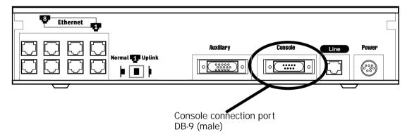
To connect the Netopia R5000 Series to your computer for serial console communication, use the supplied dual console cable connector end appropriate to your platform:
